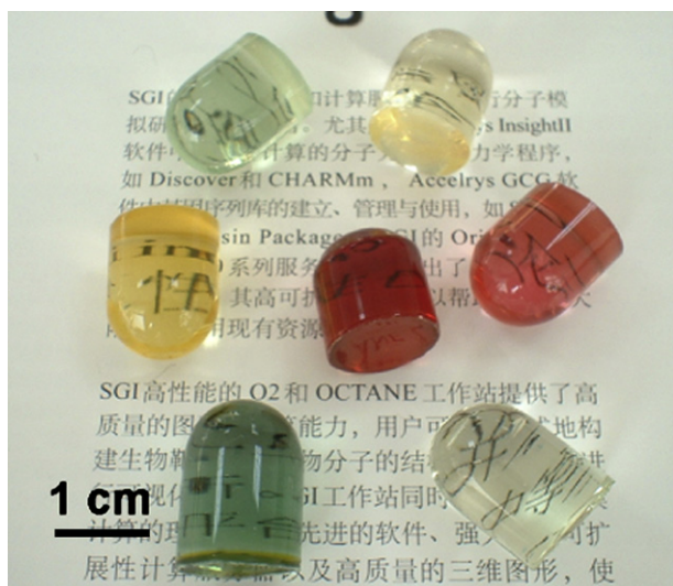
Fig. 9. Photos of the columnar SEC/PMMA composites containing different colored SECs.
